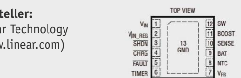
2A Solar Panel Power Manager With 7.2V LiFePO 4 Battery and 17V Peak Power Tracking
